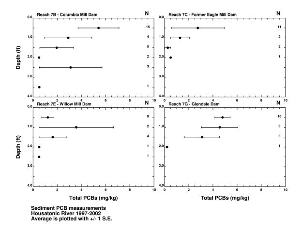
Surficial sediment PCB concentrations in Reach 7B, Reach 7C, and Reach 7G are at levels comparable to deeper sediments in Rising Pond. Remediation of sediment with these elevated PCB concentrations will remove a source of downstream transport. In addition, absent remediation of the sediments in the Reach 7 Impoundments, PCBs from the local sediment in the Impoundments which enters the water column and food chain will continue to keep fish tissue
